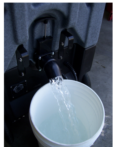
Draining the Recovery Tank
