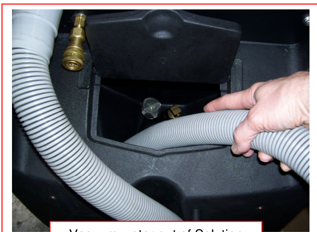
Vacuum water out of Solution Tank
